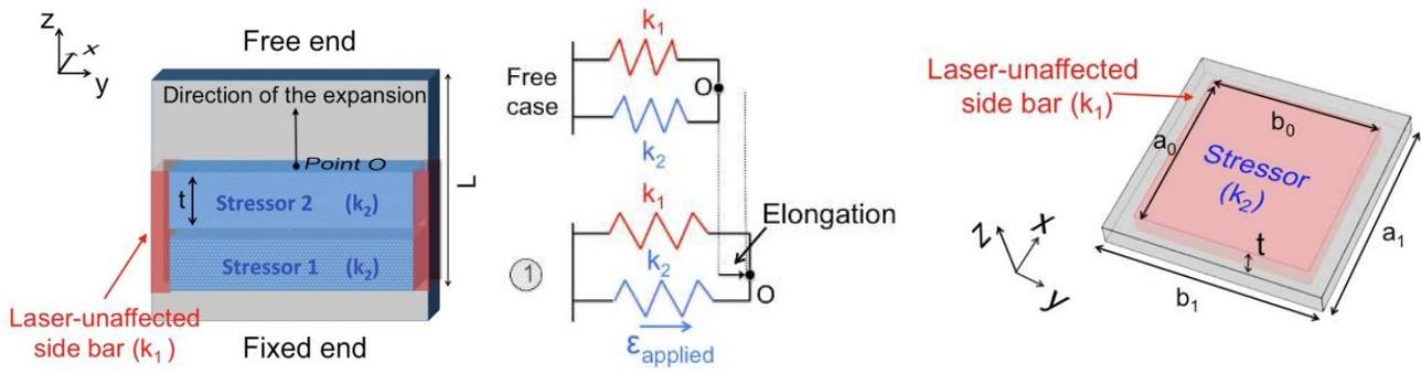
Figure 2. (a) 2D visualization of the loading process during the writing of the stressors. The mechanical energy that develops due to the localized material expansion, results in the principal loading of the sidebars. (b) Simplified spring model of the loading process. (c) Parameters used to describe a single stressor.
