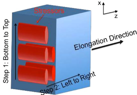
Figure 4. The writing strategy of the stressors machining along the loading bar is illustrated. Due to the built-up of internal stresses during the machining process the writing strategy plays a key role to the microstructure of the material that is formed and eventually its elastic modulus.
