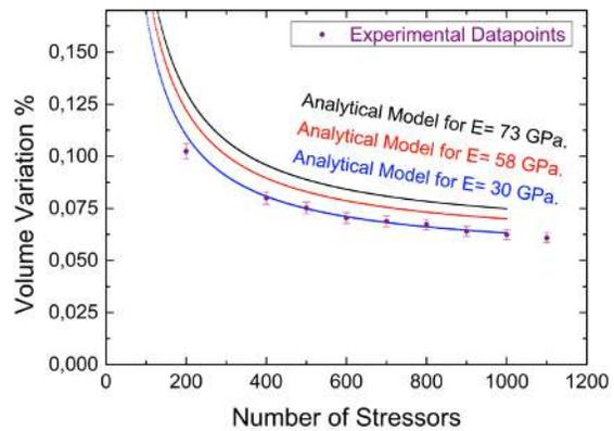
Figure 3. (a) Using white light interferometry for measuring the profile of the deformed device, a significant volume variation was found and attributed to out-of-plane motion. (b) Analytical model for different values of elastic modulus for
