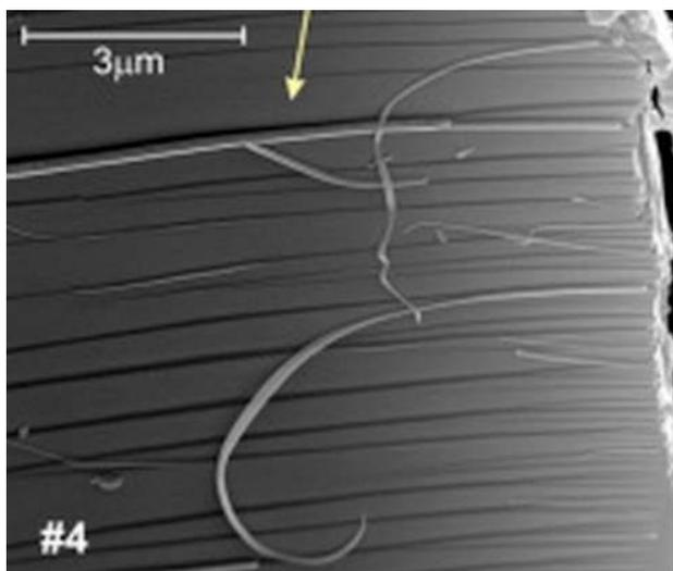
**Figure 1.** Bellouard [7] reported the evidence of localized nano plastic flow via studies of fused silica flexures under high bending stresses.
