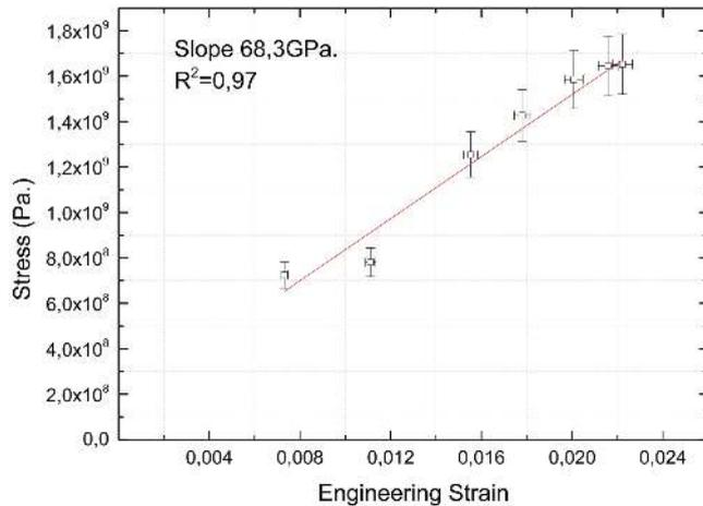
**Figure 8.** Stress vs. Strain curve of fused silica resulting to the estimate of the elastic modulus using a first order model of the mechanism.
