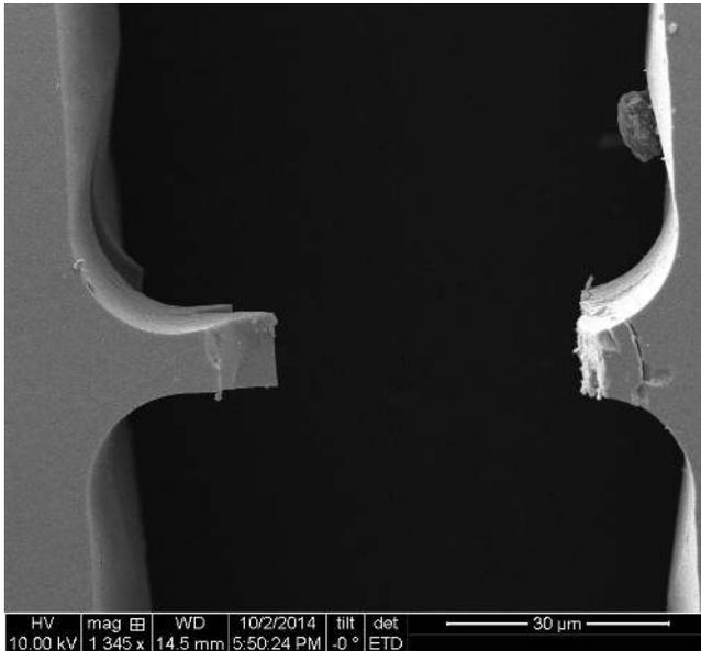
**Figure 9.** Scanning electron microscopy image of the test beam after its failure. The test beam failed for a stress between 1,7 GPa. and 1,8 GPa.
