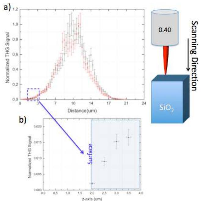
**Figure 5.** (a) THG scanned signal acquired by crossing vertically the surface of a test sample (b) The sharp transition of the acquired signal helps us define easily the surface of the sample.
