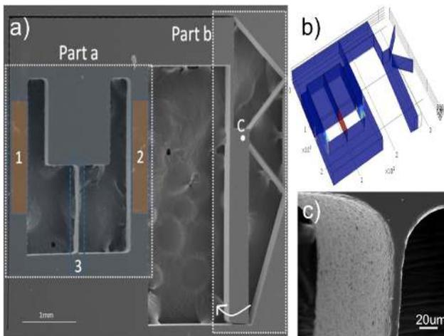
**Figure 2.** (a) Micro-tensile tester scanning electron microscope image. The overall dimensions of the system are  $2.5\text{ mm} \times 2.9\text{ mm}$ . Part a is the loading cell while part b is the displacement amplification sensor. (b) A finite element analysis image for the system loaded is shown. (c) Magnified view of the dog-bone specimen. The rounded corners are designed as such to minimize stress concentrations in the test beam.
