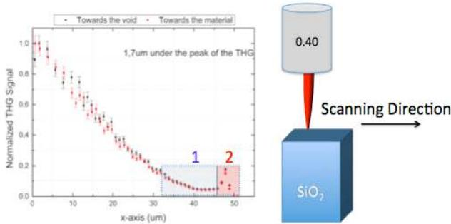
**Figure 6.** THG scanned signal across the edge of a test sample. In region 1 there is a decay of the signal while region 2 indicates a small spike thanks to which we can perform subsurface edge detection.
