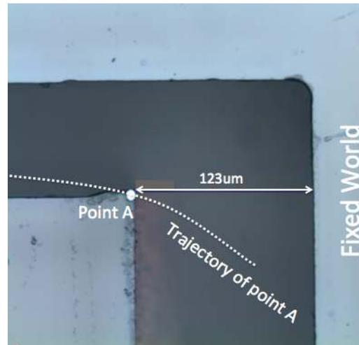
**Figure 4.** Optical microscopy image of the output of the displacement's amplification sensor. The displacement is measured as the distance of point's A trajectory in respect to a fixed point. This displacement corresponds to the actual strain of the test beam.
