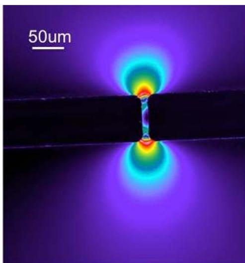
**Figure 3.** Retardance false colour map of the test beam. The stress is uniformly distributed in the beam. The highest stress is found in the regions close to the attached parts of the beam with the specimen.
