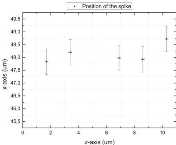
**Figure 7.** Position of the spike when scanning in different depths of the material. Therefore, there is the capability of the THG to perform subsurface edge-detection.
